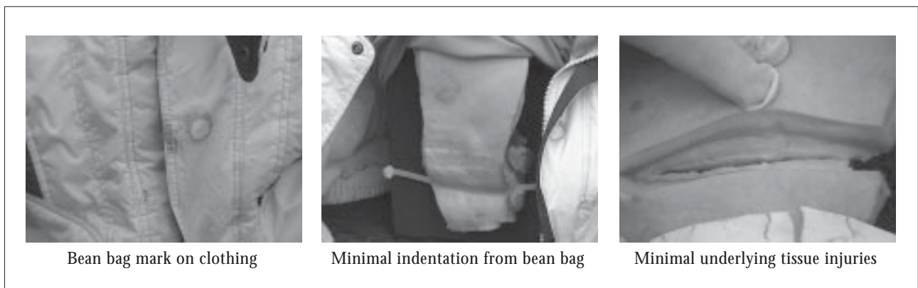
Figure 5. Results of 5 meters range shot on pork rib with heavy clothing.
