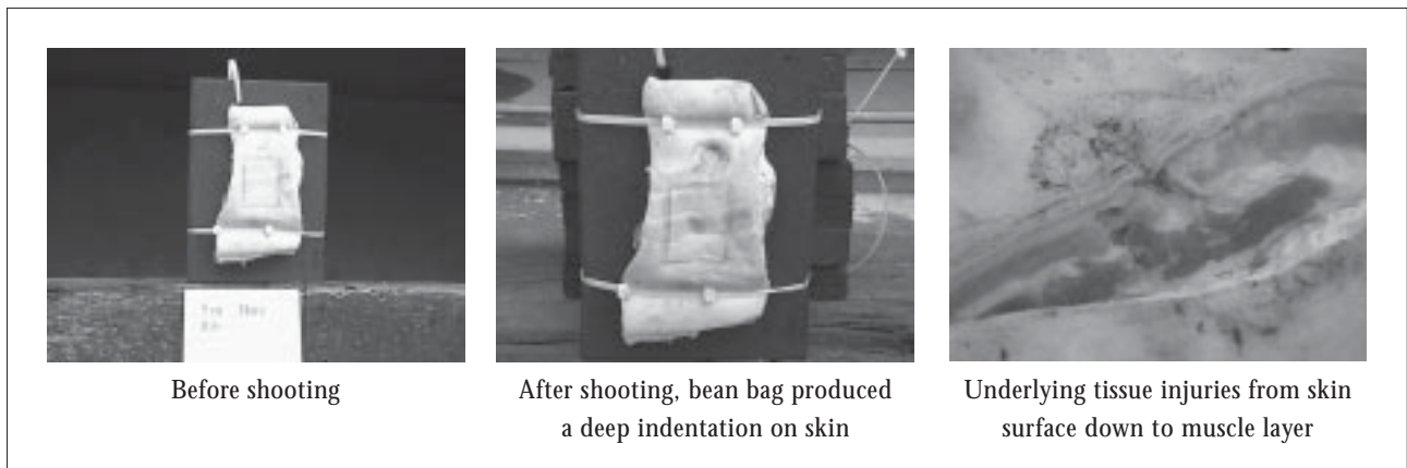
Figure 3. Results of 5 meters range shot on bare pork rib.
